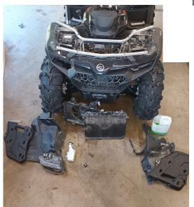
1. Remove the front luggage rack covers, wheel arch liners, radiator with fan. Remove the expansion tank and horn.
