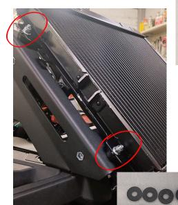
In the KIT you will find: M6x30 Bolts 4pcs 6x18 Black Washers 4pcs M6 Nut 4pcs Connect the 6mm transparent hose to the expansion tank and radiator filler neck.
