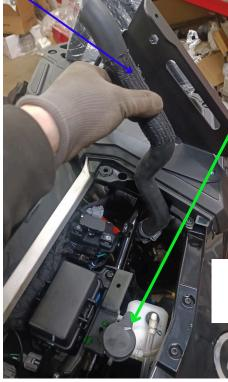
Fill the expansion tank with coolant to the MAX level.
