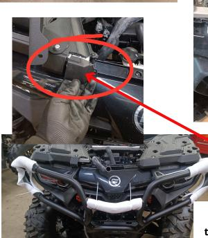
3. Mount the front bar and the plastic end covers of the luggage rack. Cut off the right corner of the plastic as shown in the picture.
