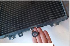
Cut off the original horn mounting bracket from the radiator.
