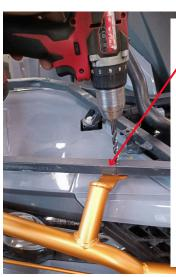
Drill an 8.5mm hole in the metal part of the package frame and then also in the plastic. Drill only through the upper surface of the tube, below it is a bushing with an M8 thread. This thread needs to stay useable.
