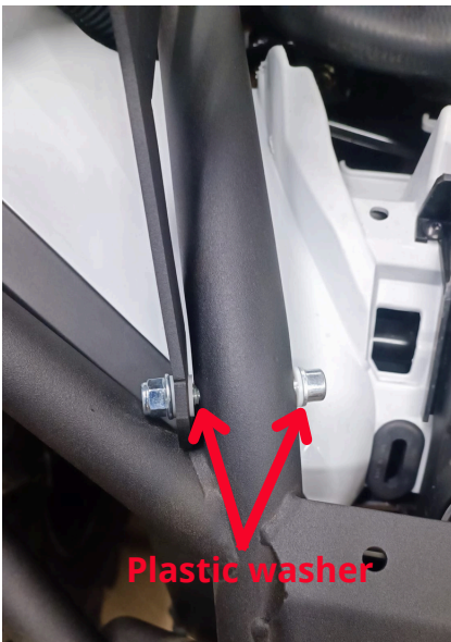
Side frame front mount. M8x60 bolt, metal washer, plastik washers and nuts
