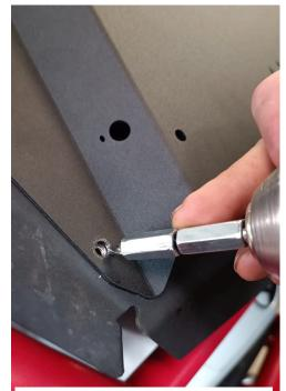
Carefully drill 5mm holes. using a drill with distance bushings. Once the holes are drilled, use a 6mm threader and thread carefully.
