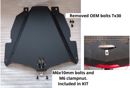
Install the scope with three original torx bolts, don't tighten it all the way right away!
