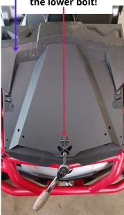
Remove the top plastic cover and tighteen these torx bolts also.
