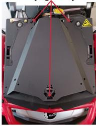
Install the top plastic cover. Set the scope in the center and tighten the lower bolt!
